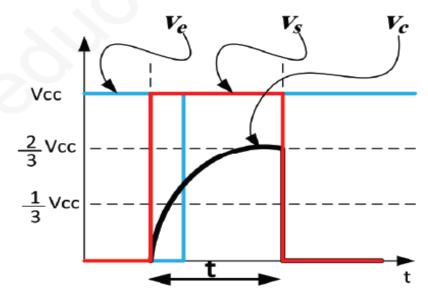
$$V^-=rac{V_{cc} imes R_2}{R_2+R_1}$$
